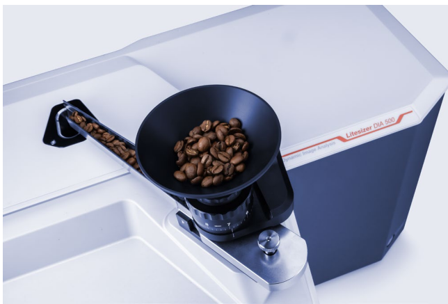
Figure 2: Whole coffee beans can be analyzed thanks to the Free Fall dispersion's large-sized vibratory hopper and chute.
